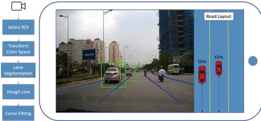
Figure 3: a (Left) Flowchart of our solution and b (Right) Results of multiple lane detection, vehicle detection and vehicle-to-vehicle distance estimation are implemented in mobile platforms.
